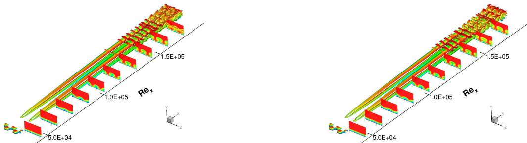
Fig. 2. Isosurfaces obtained with Q = 0.5 colored by temperature (\theta) and the temperature distribution over a z \times y slices.
