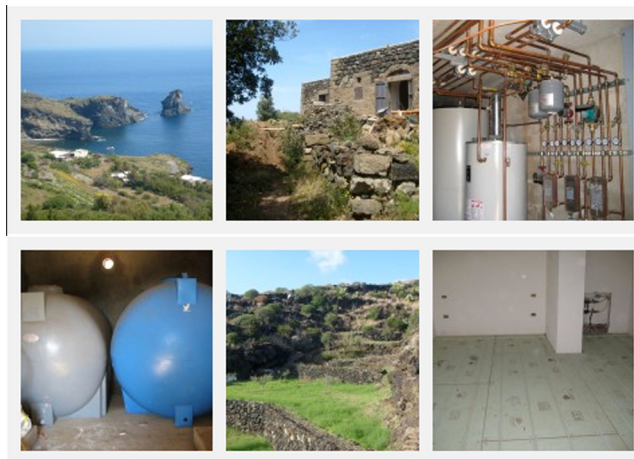
Figure 5. Images of an historic home refurbished in 2010 in Pantelleria, whose energy needs are met using solar energy. Solar hot water provides the domestic via a radiant floor heating, with ground water collected from the dome shaped roof and stored in a cistern built in the 12th century. [Reproduced from sustainabledesignpm.com, with kind permission.]
