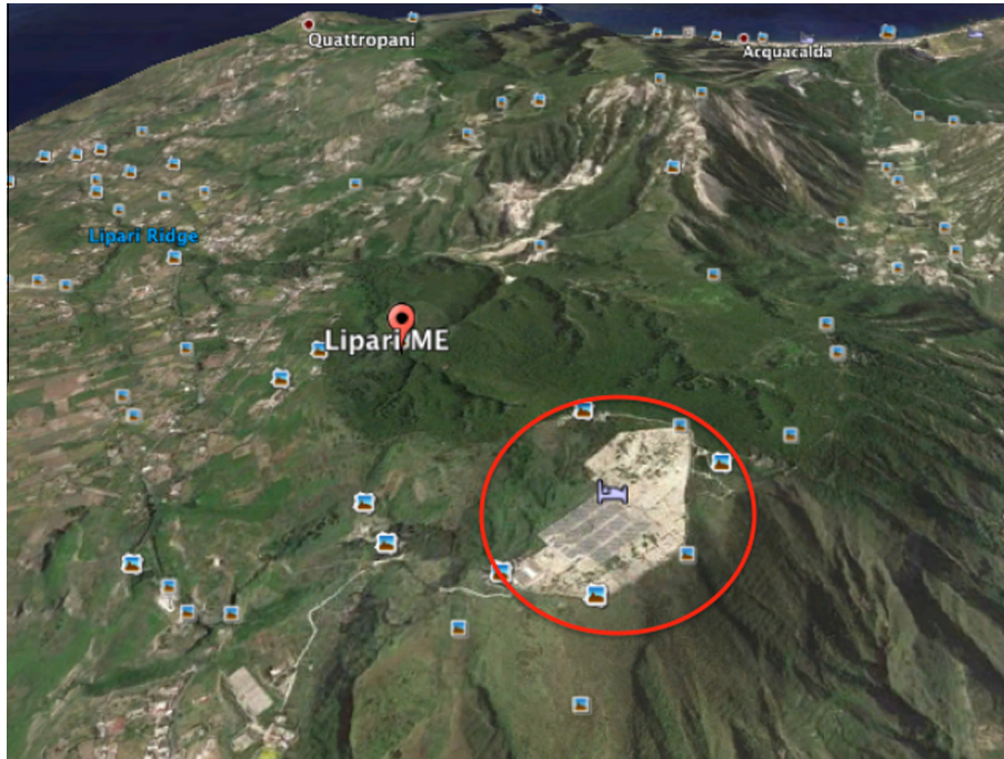
Figure 3. 1.12 MW photovoltaic field in the island of Lipari (circled in red), currently supplies most of the power needed by the new reverse osmosis desalination system installed close to the PV field. [Image obtained by the Authors with Google Earth.]
