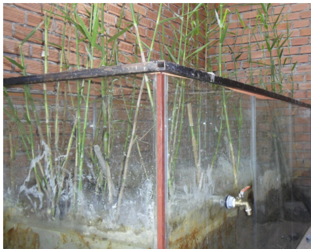
Fig. 1. Surface flow constructed wetland set-up.
