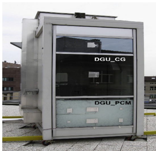
Fig. 3. DGU_PCM (bottom) and DGU_CG (top) assembled on the outdoor test facility [20]
