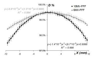
Conclusion: The factor  $K_{icdg}$ , which can be approximated by  $P_{vol}$  within 0.1 %, corrects for a dose error up to -0.6 % in reference dosimetry of the 10 MV-FFF photon beam when a Farmer ionization chamber is used.
