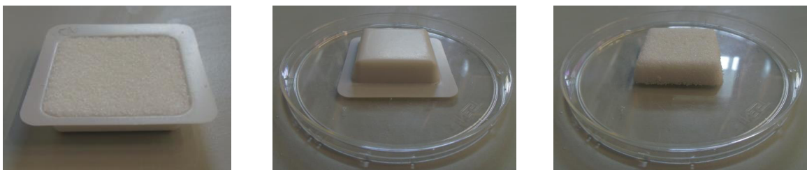
Figure 4: Lactose powder molding into weighing cup for the experiments.
