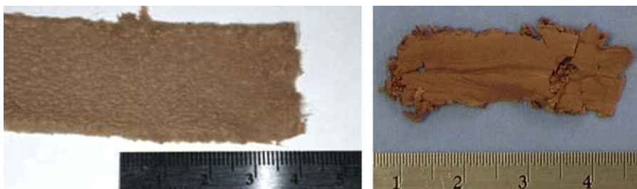
Fig. 22. Electrospun Hemoglobin and myoglobin mats using 2,2,3-trifluoroethanol solvent [115B].
