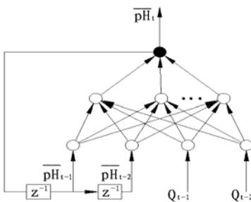
Fig. 1. ERNN network structure of pH predictive control system
