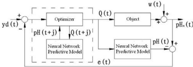
Fig.2. Neural network predictive control structure diagram
