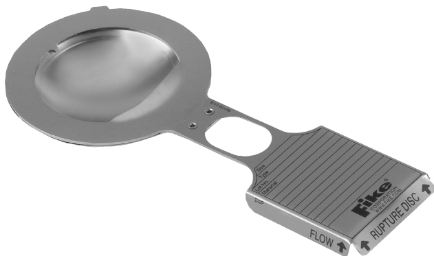
Fig. 5. The reverse buckling type rupture disc (the dome points towards the fluid under pressure) is similar to the one installed on the incident storage tank. Proper flow direction of pressure release is marked on the nameplate. (Photo courtesy of Fike Corporation.)
