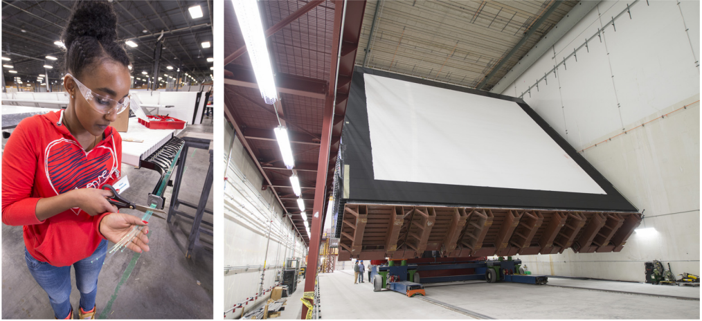
Fig. 2. Left: A student trims excess wave-length shifting fiber from the end of a 32-cell NOvA module at the factory at the University of Minnesota. Right: A single block of the NOvA detector is moved into place at the FD laboratory. Photo credits: Reidar Hahn, Fermilab.
