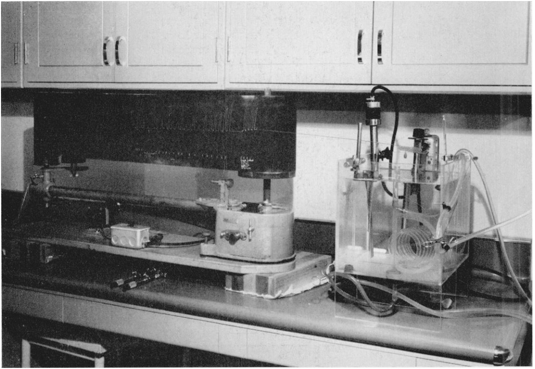
FIG. 3. Equipment for bioassay of histamine and kinins.
