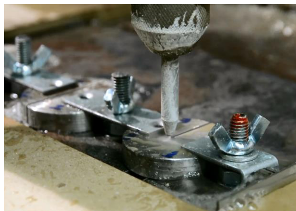
Fig.1. Abrasive water jet cutting process with experimental sample mounted in the holder.
