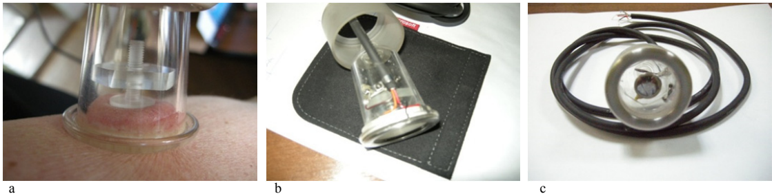
Fig. 1. Therapeutic head for combinational treatment comprising vacuum cup (a) cylindrical piezoelement (b) and RF electrodes (c).
