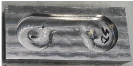
Fig. 9 Specimen machined with the archetype toolpath.
