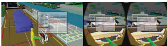
Figure 4: Mixed reality assessment system: Exo-perspective on powerwall (left) and first person perspective rendering with menu in 3d space (right)
