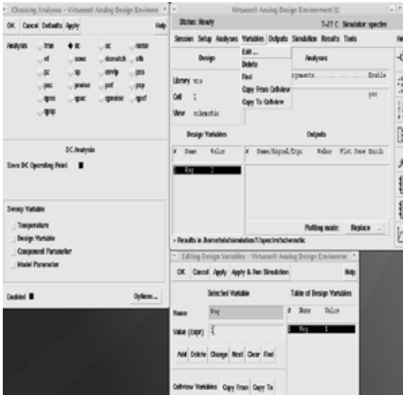
Fig. 3. Variable and dc operating point setup
