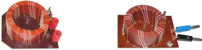
Fig. 2. The measured cores W435-04 and W516-02, Vitroperm 500F, Vacuumschmelze, Germany
