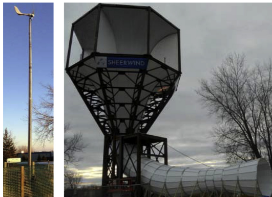
Fig. 7. Fielded INVELOX demo (right) and conventional turbine-tower system (left) under evaluation in Chaska, Minnesota.
