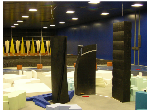
Figure 2 Boundary-layer wind tunnel test setup of the tower and its surrounding. The surrounding structures within a radius of 500 m from the center of the tallest building were modeled on the turntable.
