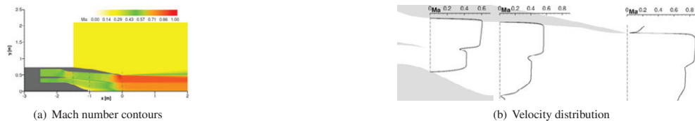
Figure 3: Base flow field obtained by a preceding RANS simulation and liner
