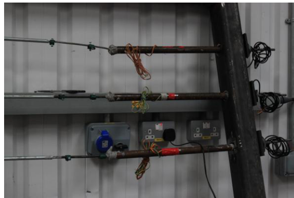
Figure 7. Samples in the Creep Rig before applying load
