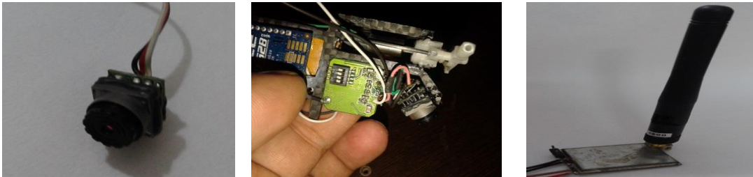
Fig. 9. (a) On-board camera; (b) FPV transmitter board; (c) FPV receiver board
