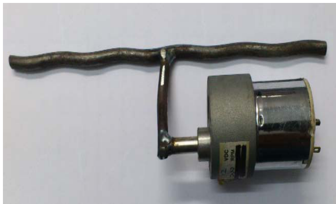
Fig. 3. DC Motor welded together with the shaft
