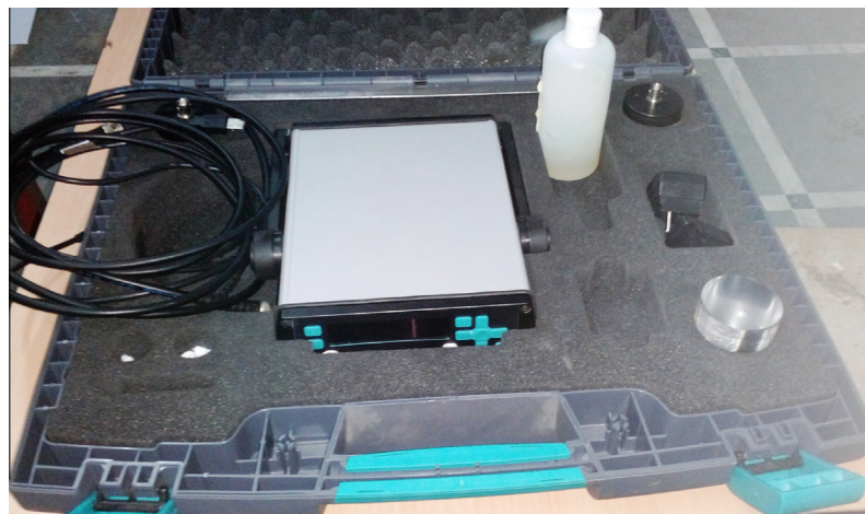
(a) UPV Apparatus
