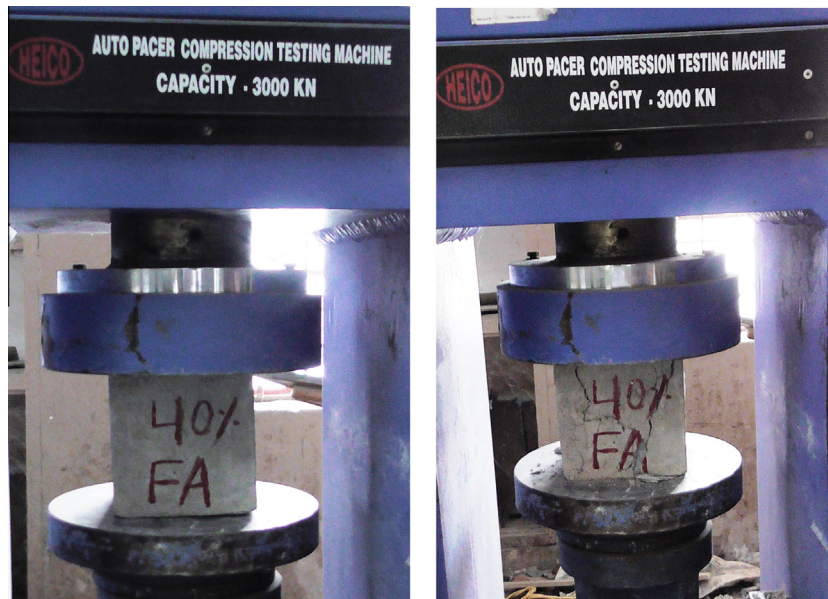
Fig. 5. Compression test (before and after test).
