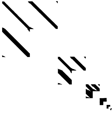
FIG. 12. The NS-form of LU factors for Example 1. The factors are combined together as \hat{T}_0 & \tilde{T}_0 and entries above the threshold 10^{-7} are shown in black.
