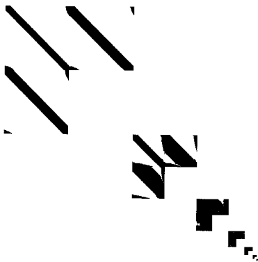
FIG. 14. The NS-form of LU factors for Example 4. The factors are combined together as \hat{T}_0 & \tilde{T}_0 and entries above the threshold 10^{-7} are shown in black.
