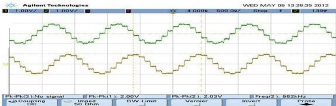
Figure 5. Output of DDS after DAC
