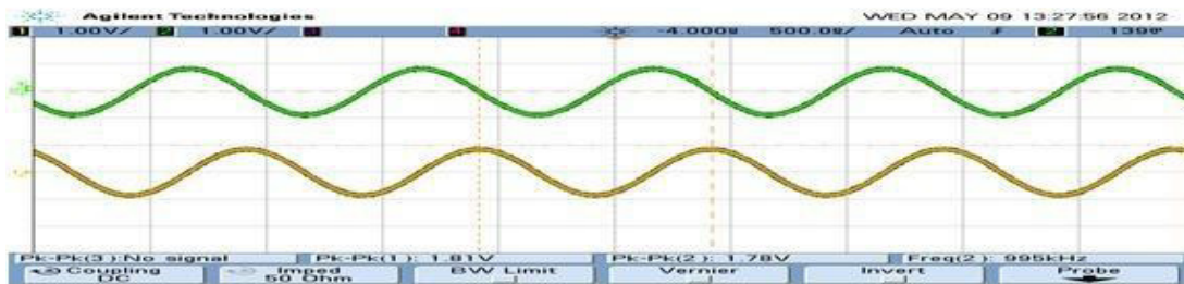
Figure 6. DDS output after DAC and LPF.
