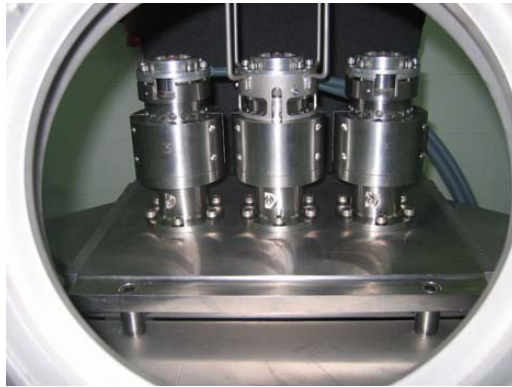
Fig. 11: Ultrasound reactor for pigment dispersion in paint manufacture.
