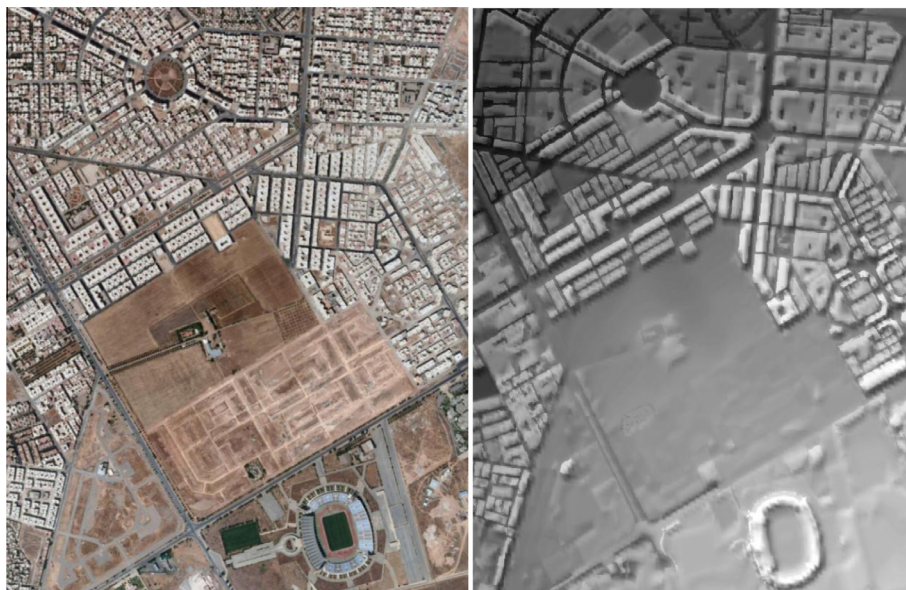
Figure 7. Orthophoto (in the left) and DSM generated from aerial photographs (in the right).
