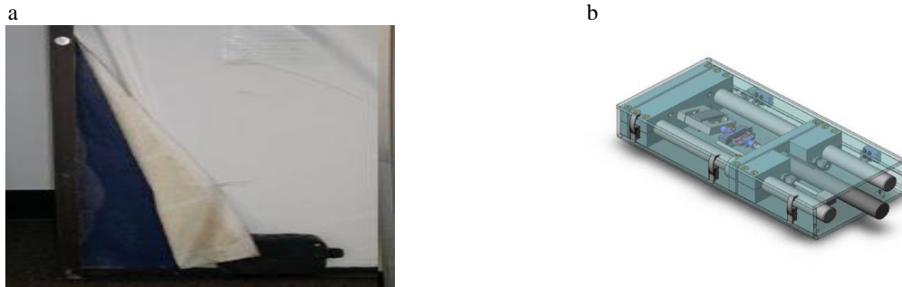
Figure 5. (a) Backsheet delamination on PV Module [17]; (b) Delamination tester [18]
