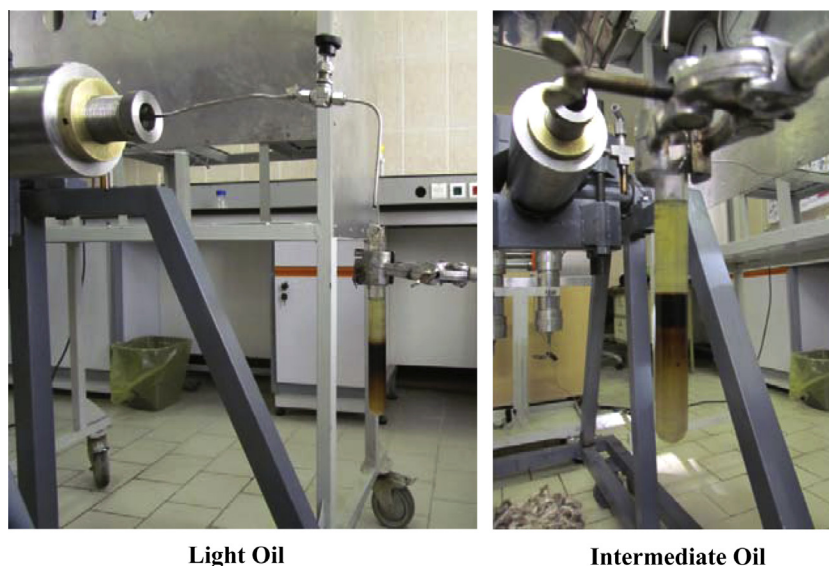
Figure 8 A schematic of produced oil after injection of nano fluid into core samples.
