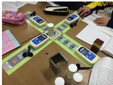
Fig.8 Measurement of radioactivity decay with distance.
