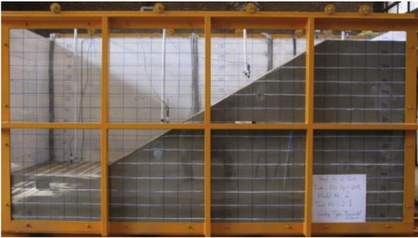
Fig. 3. Constructed physical model of slope.
