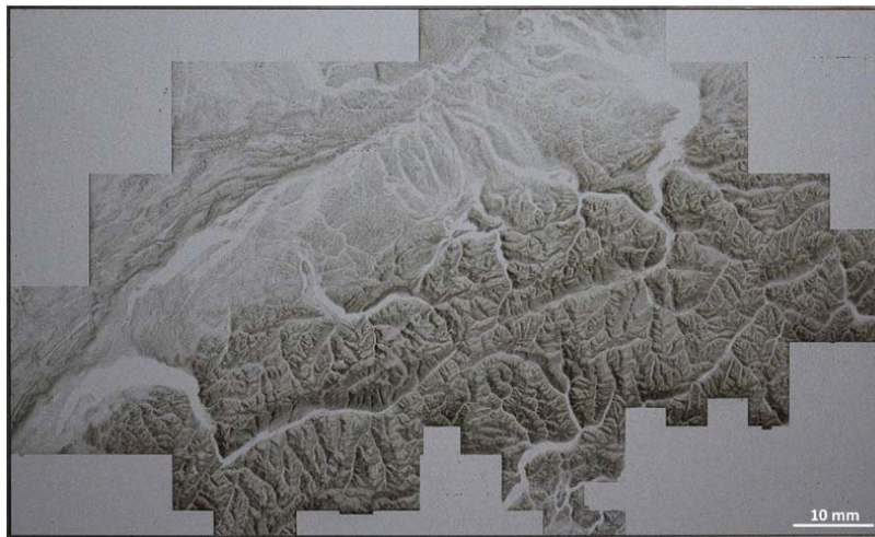
Fig. 7. Photography of the machined topography of Switzerland in stainless steel.
