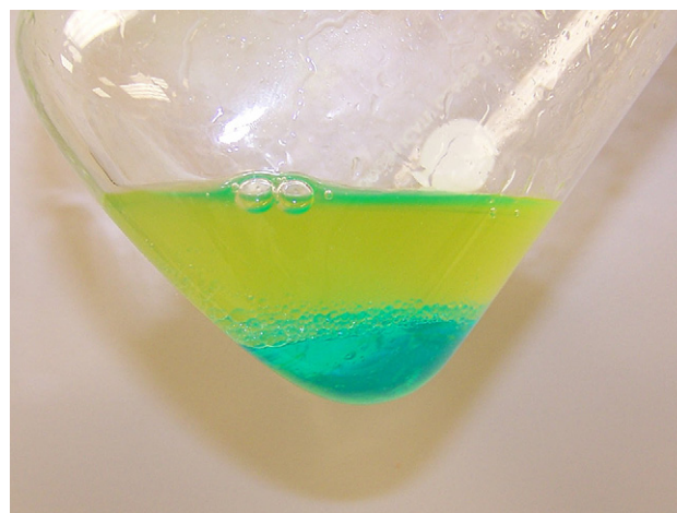
Figure 2 End point of titration the indicator turns blue.
