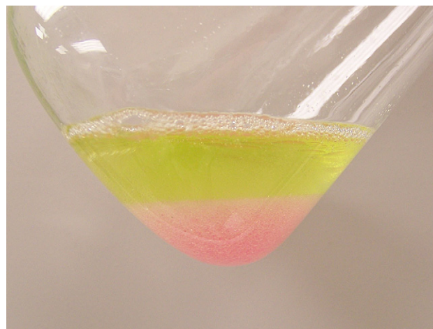
Figure 1 Start point of titration the indicator is pink.
