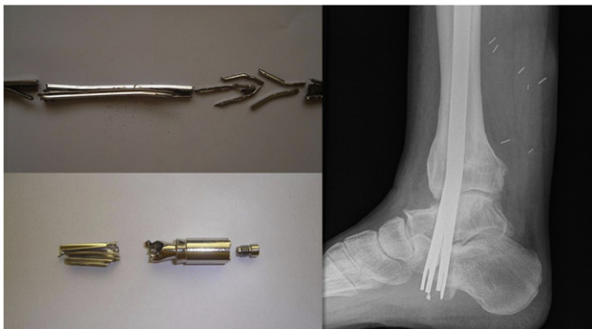
Fig. 4. Fractured nail at the junction between the valve and the metal fins.
