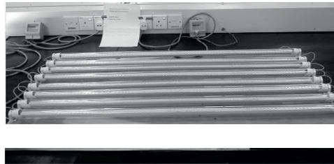
Fig. 1. LED (top) and fluorescent (below) lighting system testing setup.
