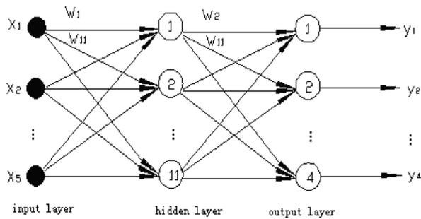
Fig..1. BP network structure chart of coal and gas outburst forecast
