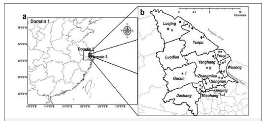
Figure 1. Two model domains for CMAQ simulation (a) and the study area (b). Circle symbols represent the 5 major industrial emission sources: 1 Baosteel Heavy Plate Subsidiary, 2 Baosteel Plant, 3 Baosteel Special Steel Subsidiary, 4 Baosteel Stainless Steel Subsidiary, 5 Huaneng Power Plant. Star symbols represent the seven monitor stations: a Baoshan Monitor Center, b Yanghang Station, c Gangyansuo Station, d Songnan Station, e Miaohang Station, f Gucun Station, a Luojing Station.
