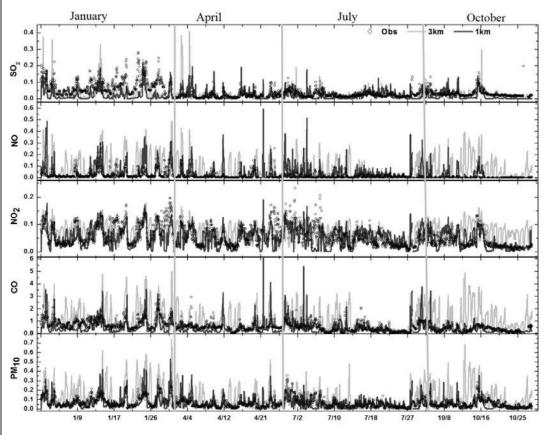
Figure 4. CMAQ results [hourly concentration (mg/m³)] at the Baoshan Monitor Center at 3 km resolution (light gray line) and 1 km resolution (dark gray line) are compared with ground observations (black circles).
