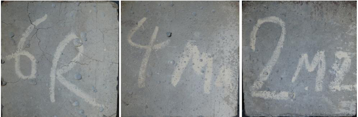
Fig. 8. Surface of tested specimens after exposure to 800°C (from left: R, M1, M2).
