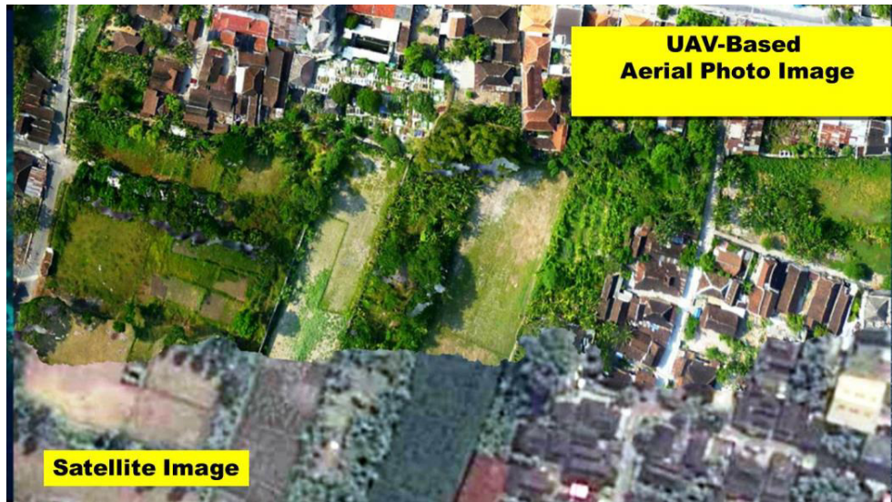
Fig. 3. Visual comparison between UAV-Based Imagery vs QuickBird satellite imagery
