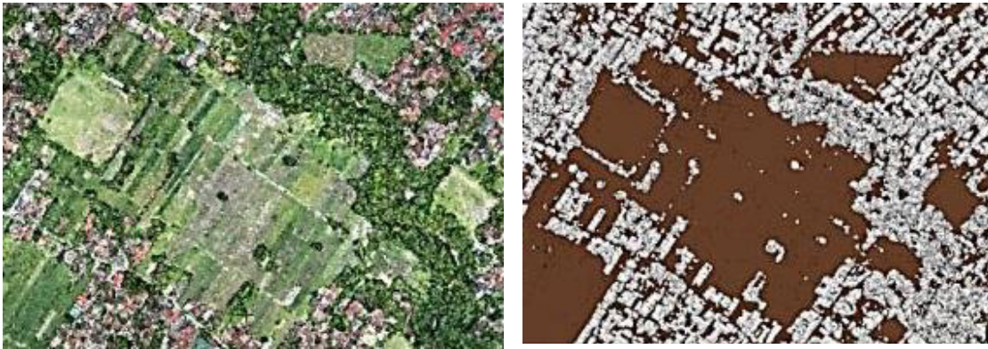
Fig. 4. Illustration of filetring process from DSM→DTM (brown)
