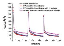
Fig 1. The flux of blank membrane, PPY and Gr/PPy modified membrane with and without applying electric field.
