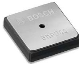
Fig. 2: BMP085 pressure sensor in an LCC-8 housing, size 5*5*1.2mm 3 , with digital output and a resolution of \pm 0.03 hPa (RMS), corresponding to \pm 0.25 m at sea level. The measuring range of 300 to 1100hPa covers -500m to +9000m above sea level. In ultra-low-power mode it requires 3 \mu A at one sample / sec., stand-by mode consumption is 0.1 \mu A. The minimum supply voltage is 1.8V.
