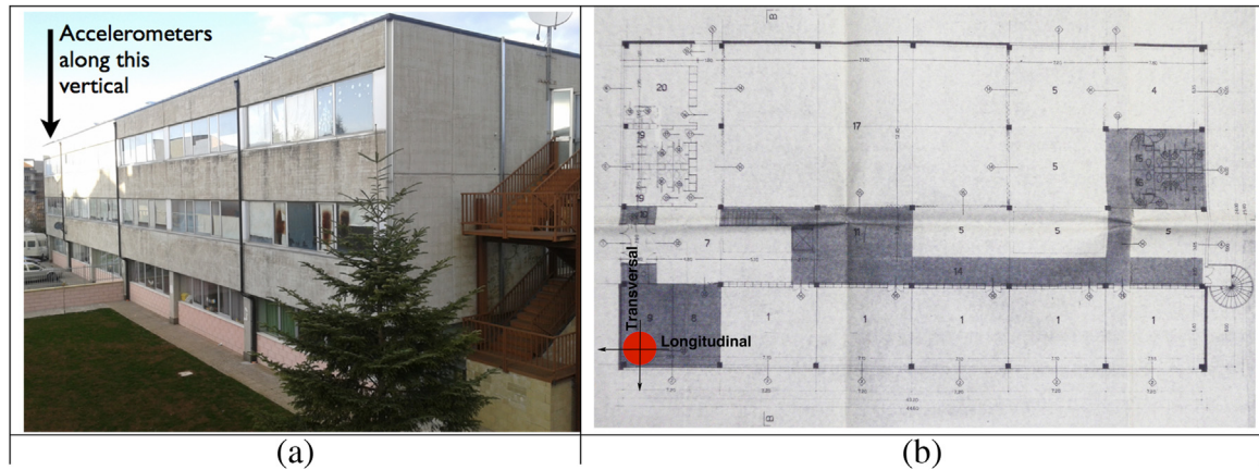
Fig. 3. (a) The building hosting the school in Rotonda indicating the vertical along which the accelerometers were installed. (b) Plan of the building indicating the position of the accelerometers (red circle) and their orientation (arrows).
