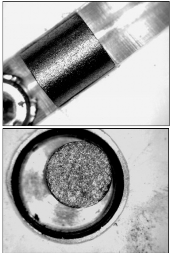
Fig. 3. Am-bearing MOX pellets fabricated for the SPHERE irradiation.
