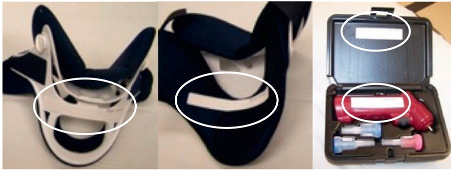
Fig. 8. Example objects with tandem tags: front (left) and back (middle) of a cervical collar; intraosseous line placement gun (right); RFID tags are circled.
