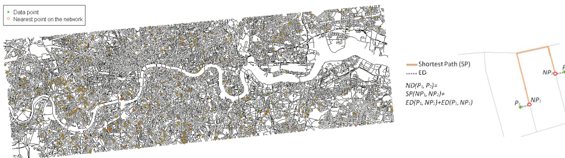
Figure 1 (a) Data points and corresponding nearest points on the given network (b) Illustration of computing ND
