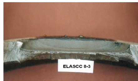
Fig. 9. Fatigued surfaces of elbows having axial notch at crown location.
