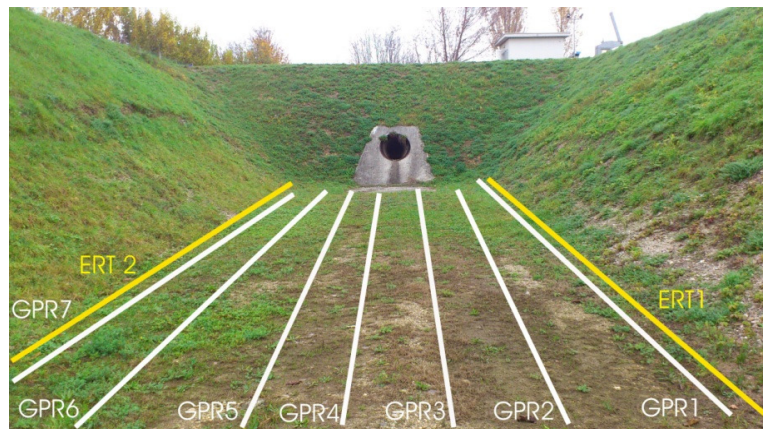
Fig. 1. Map of geophysical profiles. Seismic line is located on a road to the left out of the basin. All profiles start from inlet pipe.
