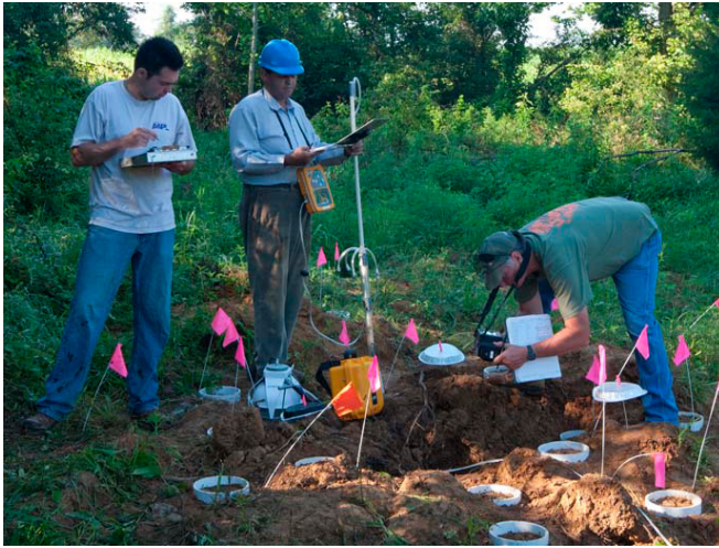
Figure 2. MVA personnel used multiple monitoring techniques to, characterize atmospheric CO 2 concentrations, soil CO 2 fluxes, and thermal signatures at the Sugar Creek EOR leak. Disturbance of the land surface was caused by the leak.
