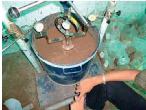
Fig. 1. The photograph of mould and Reaction frame
