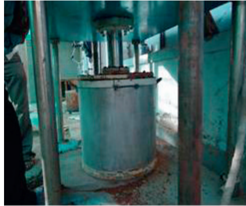
Fig. 3. Compression testing machine for static compression of sample in mould
